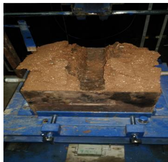
Figure3: Sample failure at 2cm rut depth
